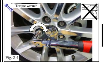
(d) Apply pressure on the key and use a torque wrench to tighten the wheel locks to 103 N·m (76 ft·lbf) (Fig. 2-4).
